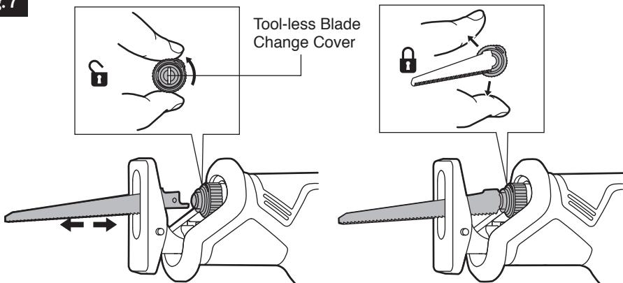
**⚠️ WARNING** Use protective gloves when removing the saw blade from the tool, or first allow the saw blade to cool down. The saw blade may be hot after prolonged use.
