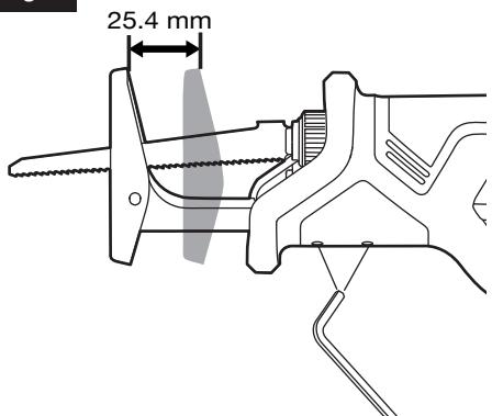
**⚠ WARNING** To avoid injury and damage, do not operate the saw without the pivot shoe in place. The blade clamp may strike against the workpiece and damage the reciprocating mechanism.
