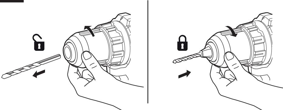
**⚠ WARNING** Use protective gloves when removing the bit from the tool, or first allow the bit to cool down. The bit may be hot after prolonged use.
