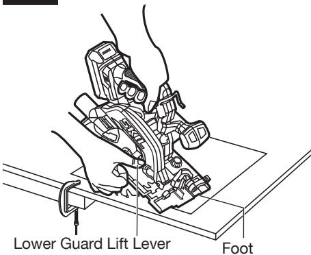
**WARNING** Allow blade to come to a complete stop before lifting the saw from cut. Also, never pull the saw backward since blade will climb out of the material and KICKBACK will occur.
