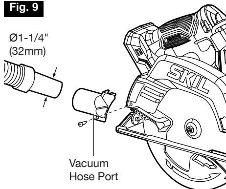
**WARNING** Never allow a vacuum/dust extractor hose to interfere with the lower guard or cutting operation.
